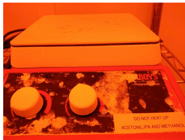
Control panel of hotplate in spin coating hood destroyed by excessive and sloppy use of (flammable!) solvents
