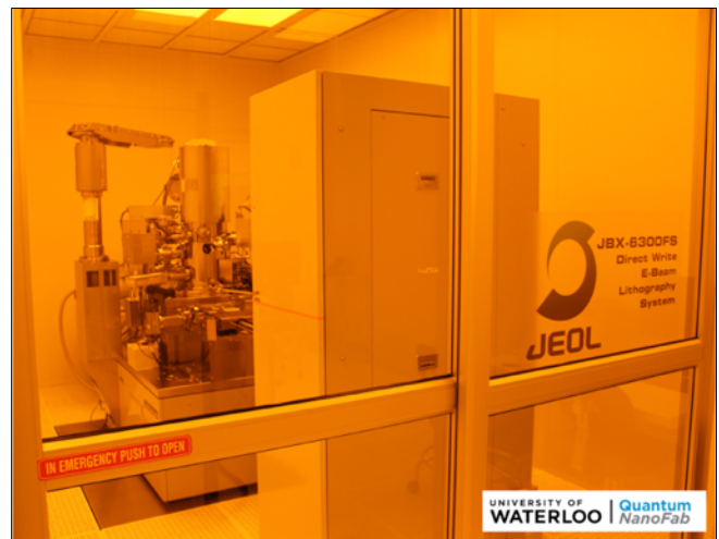
Figure 4: Fully commissioned JEOL JBX-6300FS in its new home in the Quantum NanoFab
