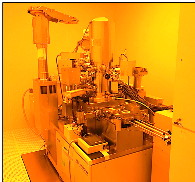
Cleanroom module 1701M housing newly commissioned 100kV JEOL JBX-6300FS Direct Write E-Beam Lithography System
